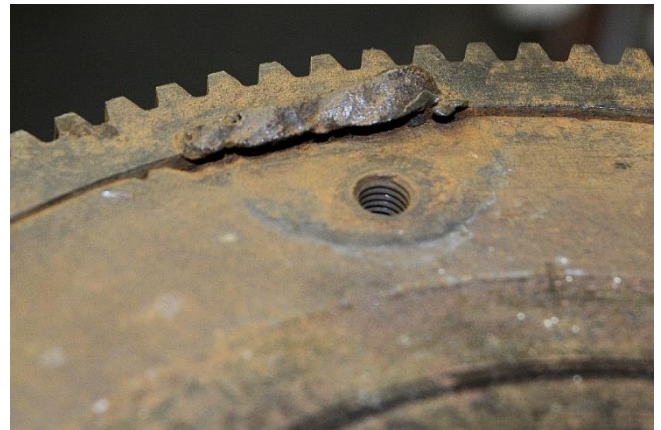
Figure 3. A close-up of a broken electric welding 'repair'.
