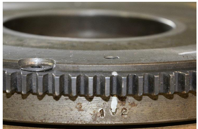
Figure 5. Detail of the carried through marking shown in white for clarity. Also visible are the spot facing of the flywheel and the countersunk setscrew face above the ring-gear face. Camera angle distorts the image.
