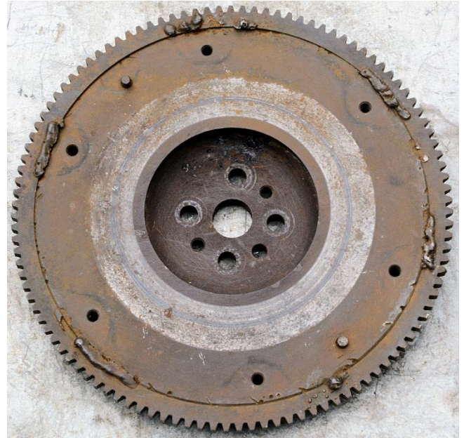
Figure 2. A graphic illustration showing how a loose ring-gear should not be repaired.
