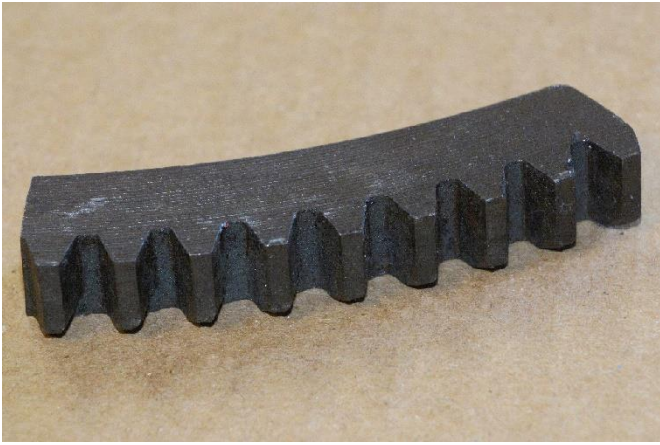
Figure 8. The piece of ring-gear for use as a wedge.
