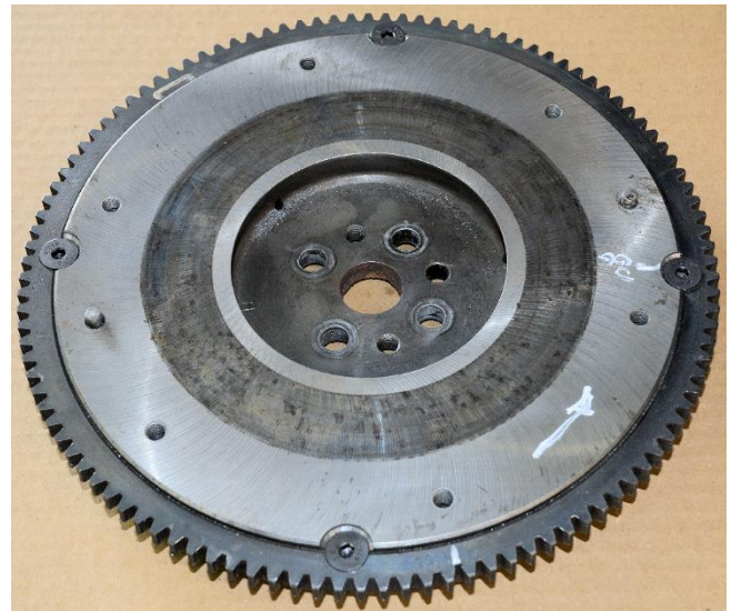
Figure 4. How the marking out commenced with the 1 and 2 TDC mark carried through to the clutch face.
