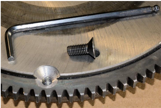
Figure 6. Showing the spot facing so that drill can start the hole at centre between ring-gear and flywheel. Also shown is extent of counter sink machining. The counter-sunk setscrew is 8 mm thread diameter with 20 mm overall length. A very good illustration of the 'scotch-key' method of securing the ring-gear.
