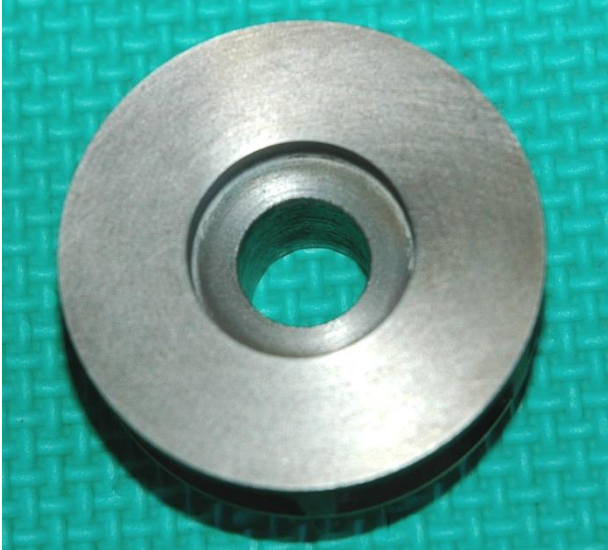
Figure 1: Rear face of impeller with machined recess.
