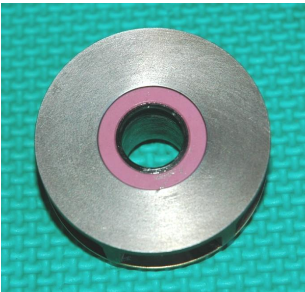
Figure 2: Showing the ceramic ring and boot in place.
