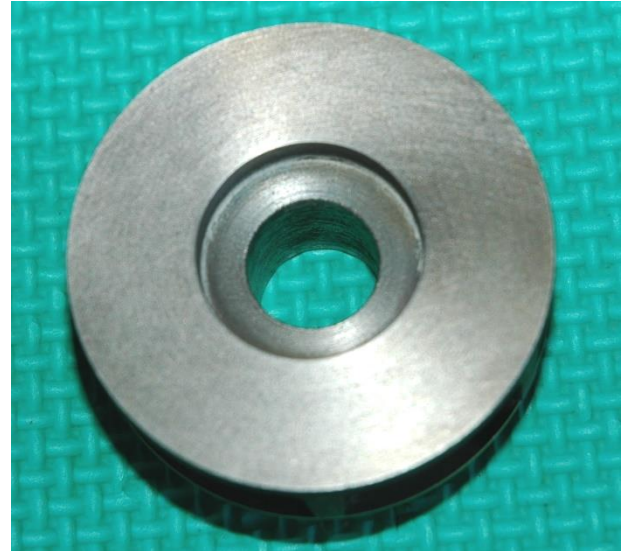
Figure 1: Rear face of impeller with machined recess.
