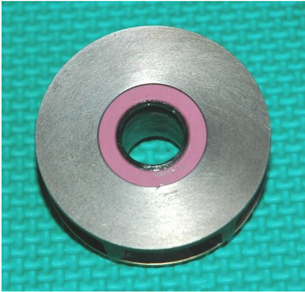
Figure 2. Ceramic ring in impeller.
