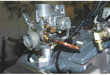
Right: A Solex carburettor mounted in position.
