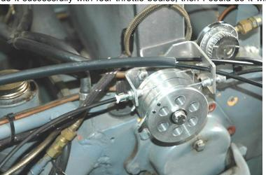
clear, the accelerator pedal had its own return spring and each Solex carburettor had its own return spring – thus, it would be but a simple matter to devise an intermediate drum, rotated by a single cable from the pedal and, have attached to the drum two precisely located cables, one for each carburettor.
