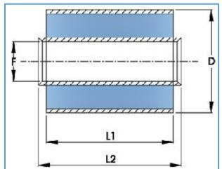
Left: Figure 2. Showing the components that make up a Silentbloc bush assembly, where 'D' is the outer steel sleeve, 'F' is the inner steel bushing and the rubber section is shown in blue.
