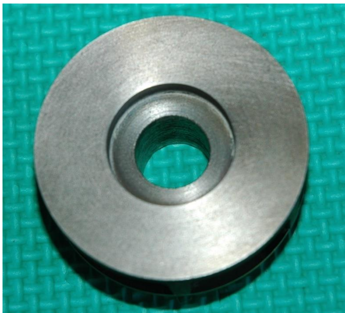
Above: Figure 18. Recess in rear of impellor.
