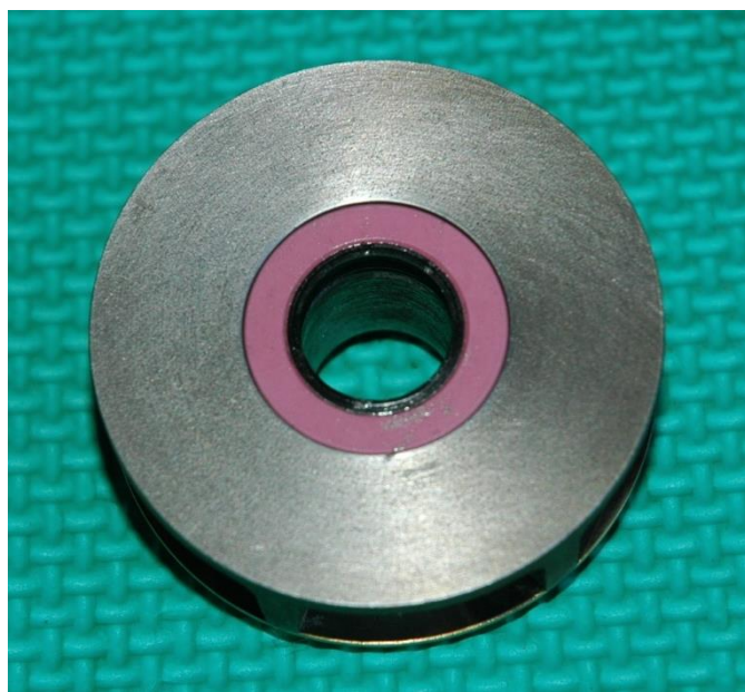
Above: Figure 19. Ceramic boot installed.
