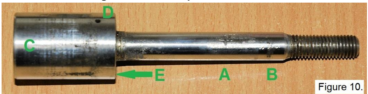
Above: Figure 10. A worn and abused plunger and rod assembly.
