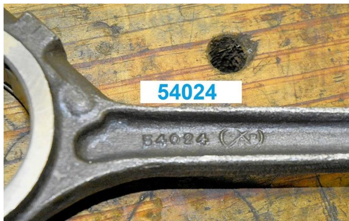
Above Left: Figure 18. Part number identification. Above: Figure 19. 'B' indicates strengthened area.
