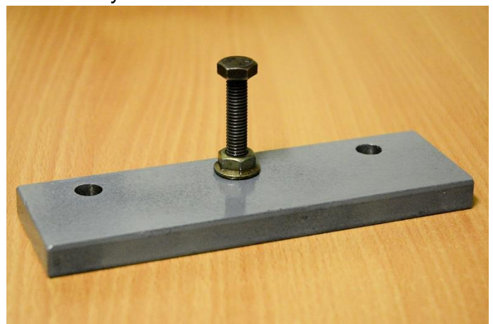
Right: Figure 23. Cylinder head removal tool.
