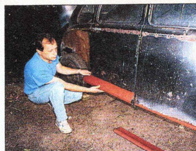
● Richard Gane offers up a JCS repair section to one of the doors on his £50 car - they are not usually that cheap!
