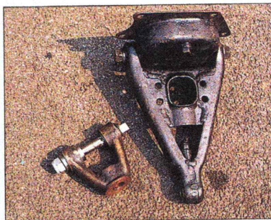
● Reconditioned bronze suspension top trunnions with oversize pins are available from Jowett Car Spares. Later types were fitted with easily replaced rubber bushes.
