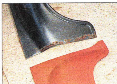
● This is where wings rot: the front along the trailing edge and the rear along the leading edge. The rear one has had a repair section inserted by Richard Gane, using his no-gas Clarkweld 100EN Turbo MIG welder.
