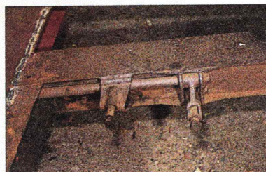
● The condition of the chassis near the front torsion bar mountings needs checking carefully. Sometimes the top of the chassis rots, allowing the bars to distort the chassis. This is difficult for the amateur to repair.
