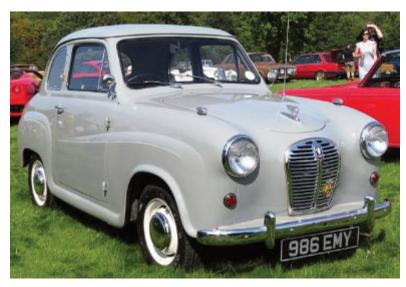
The link to the original 7 was in name only though: it was a thoroughly modern design. It was the first car produced by Austin to use monocoque construction (no separate chassis); and it also featured a new Austin designed 4-cylinder OHV engine, known as the A series. The 803cc engine developed 30 bhp – thus the name A30: Austin applied a principle of naming their cars after the power they produced.
