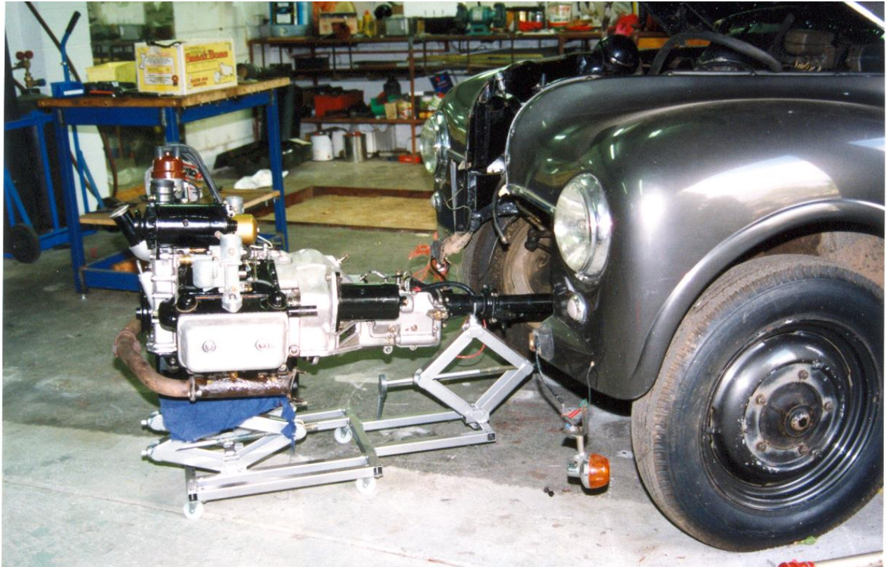
Ray Jowett's engine being installed using the purpose built engine and gearbox trolley.
