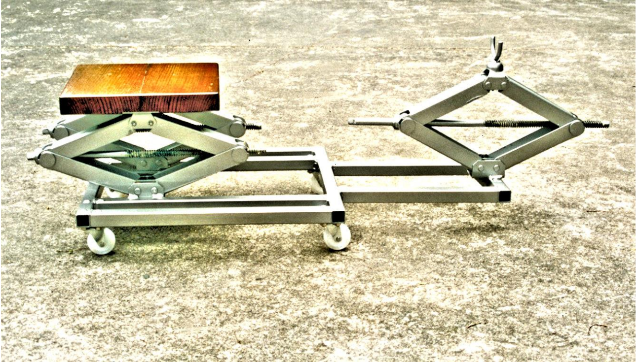
Homemade engine/gearbox trolley.
