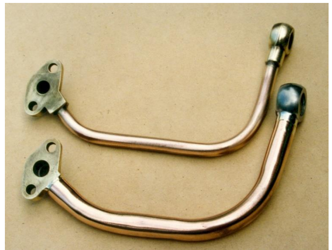
Above: Figure 11. Illustrates built up pump body. Above: Figure 12. Illustrates difference in delivery pipes. Note the smooth bend of the copper tube and how it fits over the banjo fitting and the delivery elbow.
