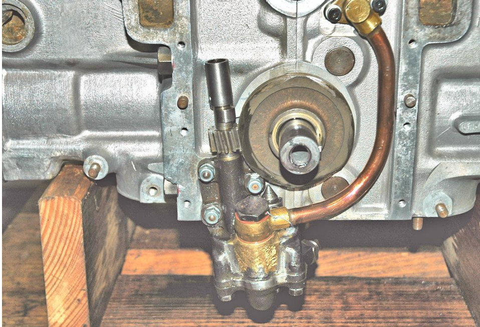
Modified oil pump, showing larger delivery pipe assembly installed on a Javelin PC crankcase. The adjustable release valve can be seen at the pump's base plate..
