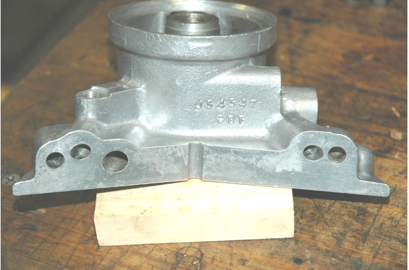
A Series III rear timing cover.
