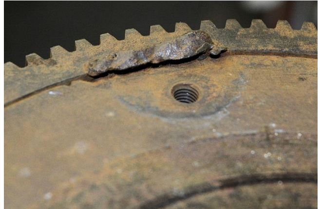
Right: Figure 3. Close-up of a broken electric welding 'repair', that has broken away.
