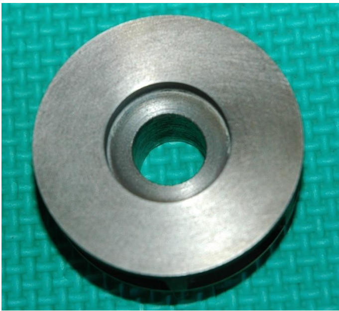
Above: Figure 18. Recess in rear of impellor.
